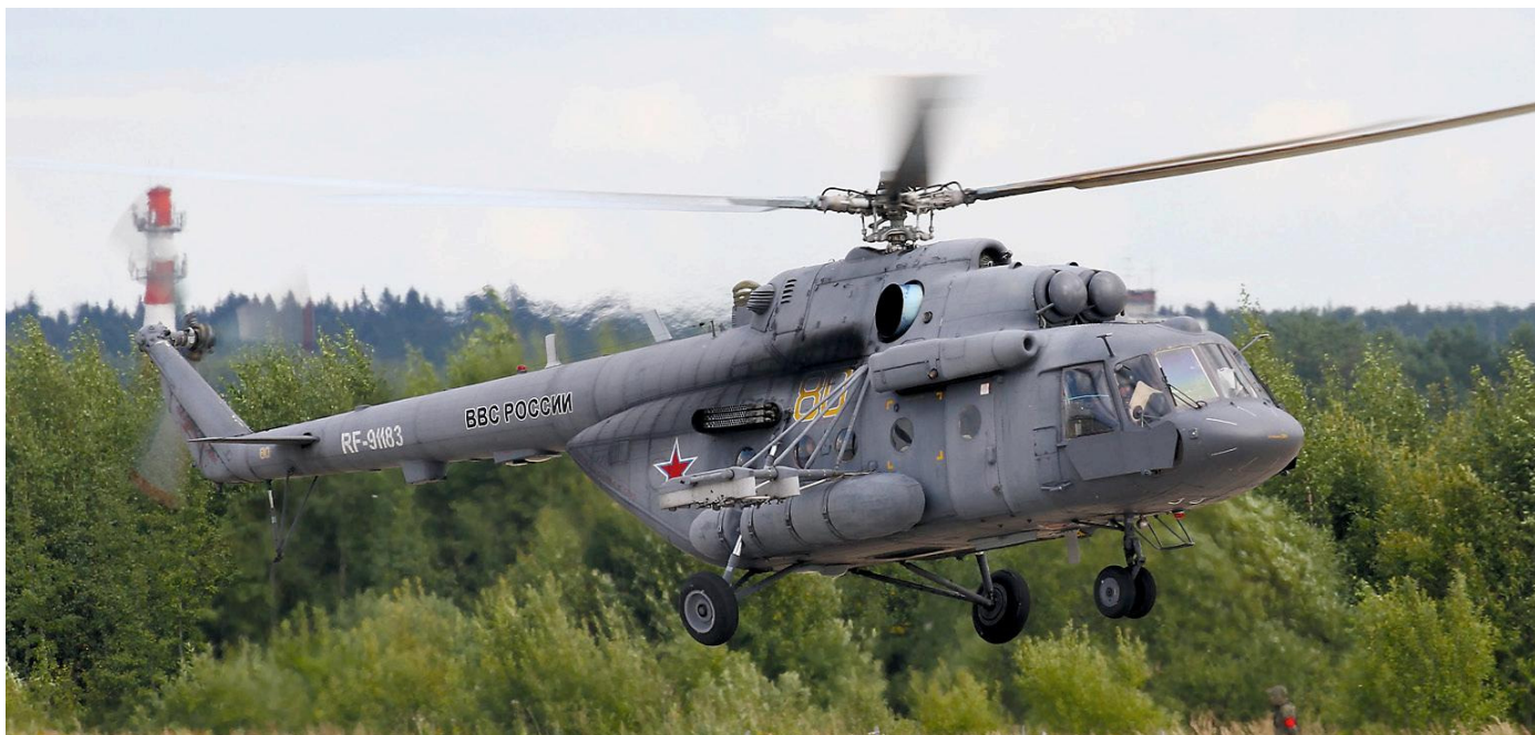
A type-recognition nightmare is the Mi-8 family. The position of the side cargo door and the bump above the cockpit reveal that this is an Mi-8MTV-5. (RF-91183/80y, 25 August 2017, Jochem Manders)
