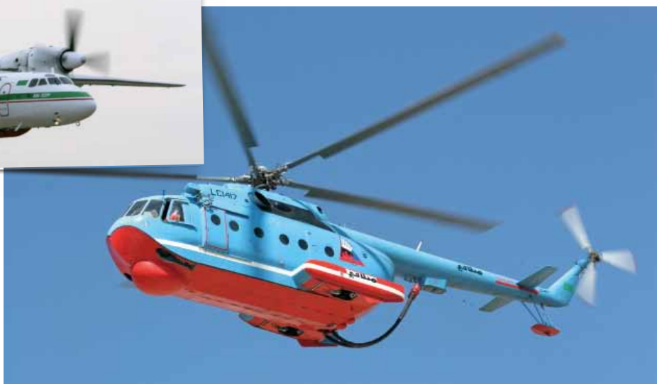
Right: Libya often suffers from fires at its gas and oil production facilities. During 2006 the LAF sent two Mi-14s to Sevastopol Aircraft Plant in Ukraine for conversion to Mi-14PZh fire-fighters, and these were returned in late 2007 and early 2008. The two hoses at the rear of the helicopter can suck some 4,000 litres of water from water only a foot (30cms) deep. They are both operated by 1014 Sqn.
