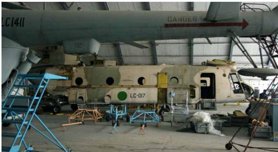
The Libyan Italian Advanced Technology Company (LIATEC) has been working with the LAF to return six Chinooks to service. The work has included installing new more powerful Honeywell T55-712E engines and the helicopter is now referred to as the CH-47C+. One example is seen here receiving attention in a hangar at Metiga during 2007.
